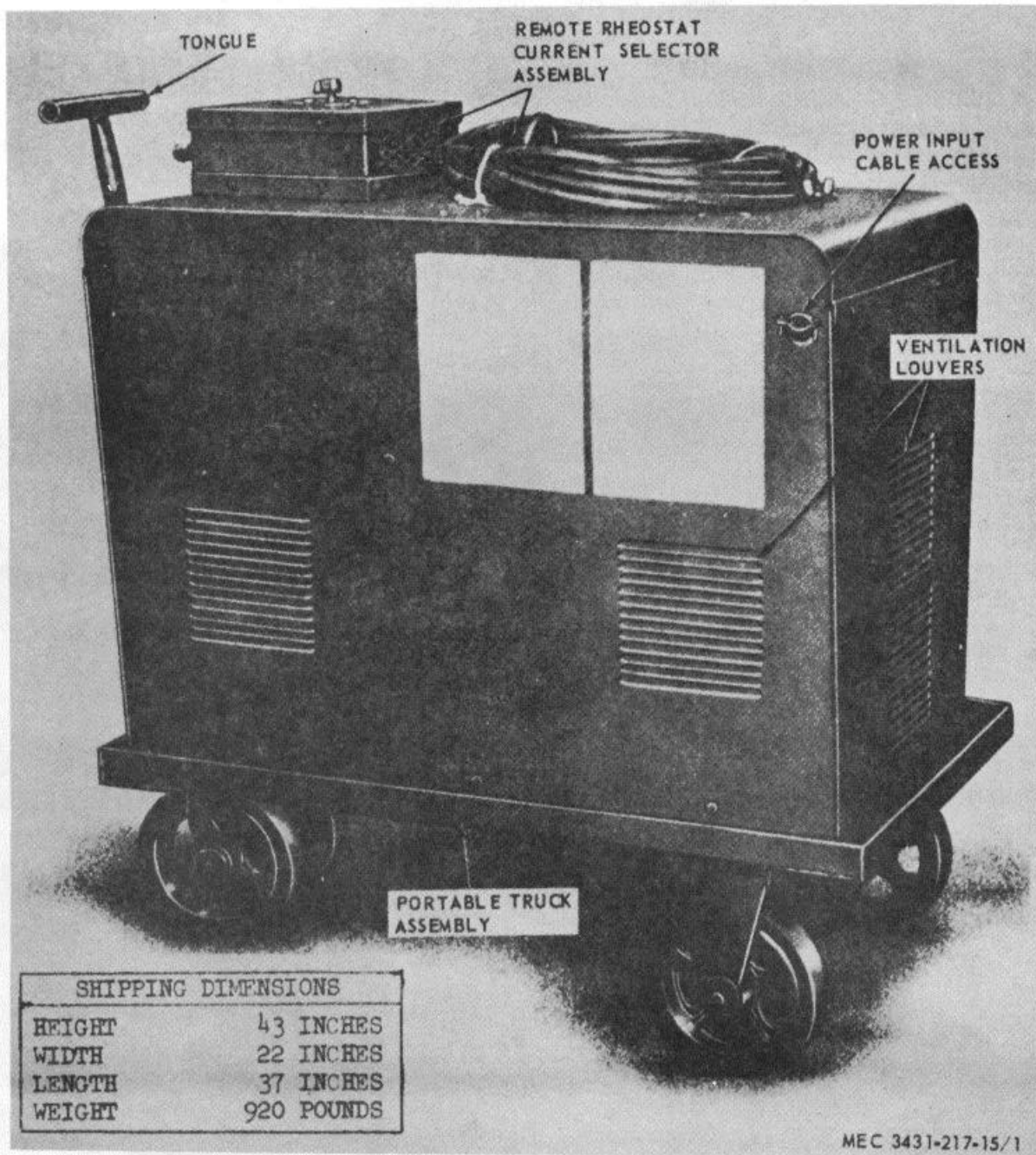
Figure 1. Arc welder rear, three-quarter view with shipping dimensions.
